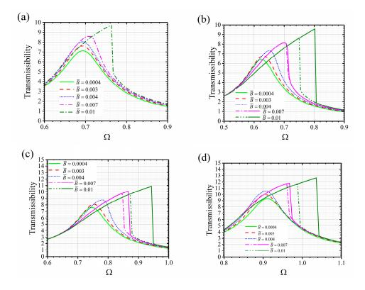
**Figure 7.** The influence of load weight on the transmissibility of the isolator. (**a**) The dimensionless load weight is 1.34. (**b**) The dimensionless load weight is 1.55. (**c**) The dimensionless load weight is 1.96. (**d**) The dimensionless load weight is 2.08.
