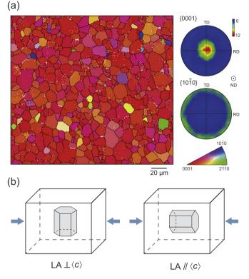
**Fig. 1.** (a) Inverse pole figure map and pole figures of rolled magnesium alloy AZ31, viewed along the normal direction (ND). (b) Illustrations of the relative orientation of the loading axis (LA) with respect to the *c*-axis.
