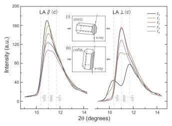
**Fig. 5.** X-ray diffraction peak intensities at instants  $t_0-t_4$  for the two loading directions. Insets: grain orientations contributing to diffraction peaks {0002} and {10  $\bar{1}$  0}.
