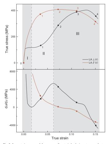
Fig. 3. Stress–strain curves and the corresponding strain hardening rate curves for two different loading directions,  $LA \perp \langle c \rangle$  and  $LA \parallel \langle c \rangle$ . The symbols (10 µs apart) denote the instants for simultaneous imaging and diffraction measurements. The curves are divided into three regimes, I–III. Numbers 0–4 represent instants  $t_0$ – $t_4$ .
