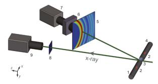
**Fig. 2.** Schematic of the experimental setup for simultaneous x-ray diffraction and imaging under high strain rate compression, along with the coordinate system (*xyz*). 1: incident bar; 2: strain gages; 3: sample; 4: transmission bar; 5: diffraction scintillator (with illustrative diffraction rings of the magnesium alloy); 6: microchannel plate; 7: diffraction camera; 8: imaging scintillator; 9: imaging camera.
