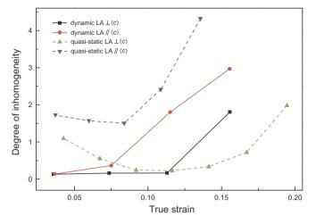
Fig. 7. Degrees of inhomogeneity of normal strain fields as a function of true strain under dynamic (solid curves) and quasi-static (dashed curves), obtained form Ref. [15].
