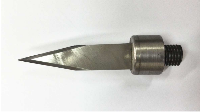
Figure S1 the engineered spike for piercing tests.
