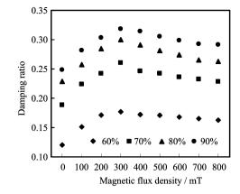
FIG. 4 Damping ratio of MR elastomers with different iron particle proportions.
