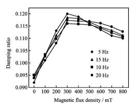
FIG. 3 Damping ratio of MR elastomers measured at different driving frequencies.
