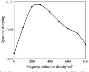
Fig.6 Change curve of dynamic damping of MRE with test magnetic field
