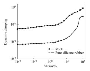
Fig.4 Change curves of dynamic damping with strain amplitude of MRE
