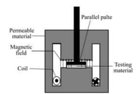
Fig.3 Principle diagram of MR-device of rheometer
