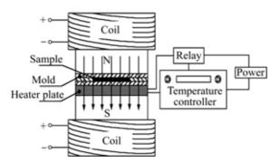
Fig.1 Schematic diagram of PS device
