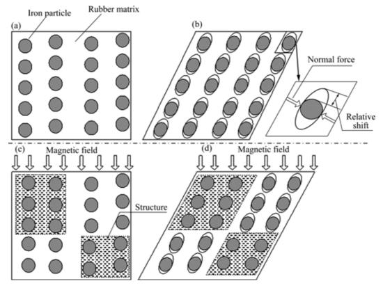
Fig.8 Schematic diagram of structures of MRE
