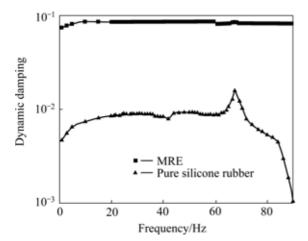
Fig.5 Change curves of dynamic damping of MRE with frequency
