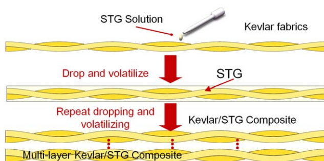
Figure 1. The schematic of the dissolution-volatilization fabrication procedure to prepare Kevlar/STG composites.
