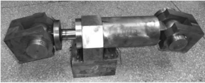
Figure 5. Photograph of the MR damper.
