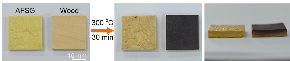
Figure S20. Optical images showing the morphologies of AFSG and poplar wood after heating at 300°C for 30 min. The wood has severe surface carbonization along with bulking while AFSG remained almost intact.
