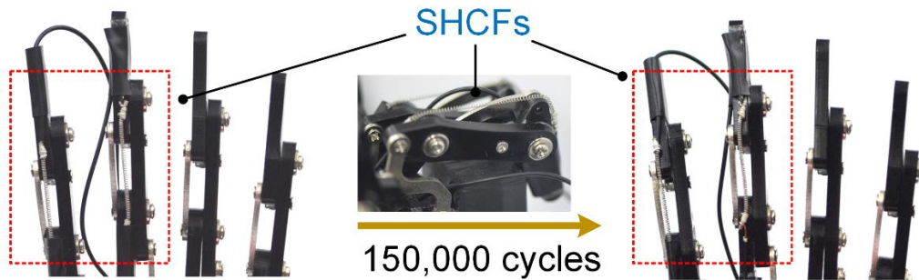
Figure S21. Morphology changes of SHCFs after 150 000 cyclic bending.
