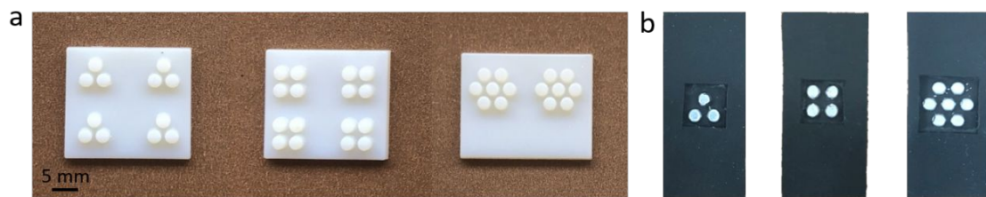
Figure S2. (a) Optical photographs of different kinds of 3D printed molds and (b) the as-fabricated H-LMDE composites with different arrangement of droplets.
