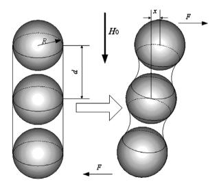
Fig. 2. The shear model of particles chain.
