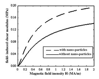
Fig. 3. The predicted field-dependent shear modulus.
