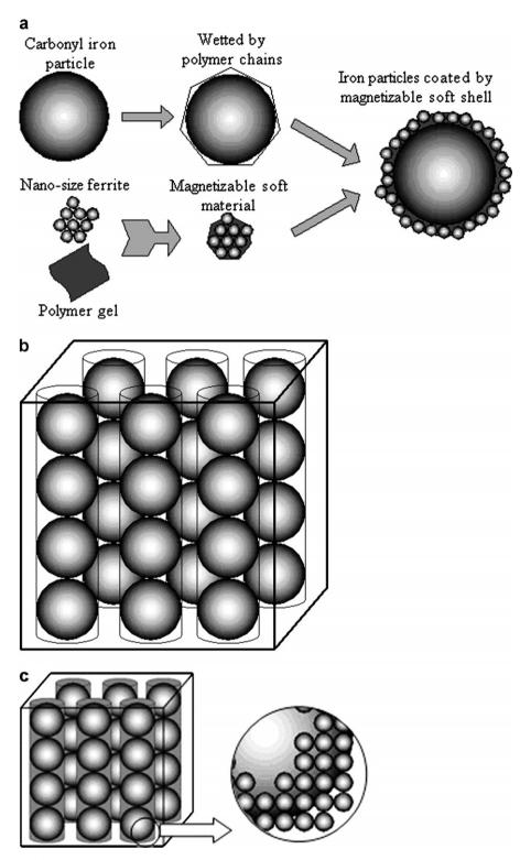
Fig. 1. New construction MREs: (a) Fabricate process, (b) traditional MR elastomers construction and (c) MR elastomers with nano-size particles additive.
