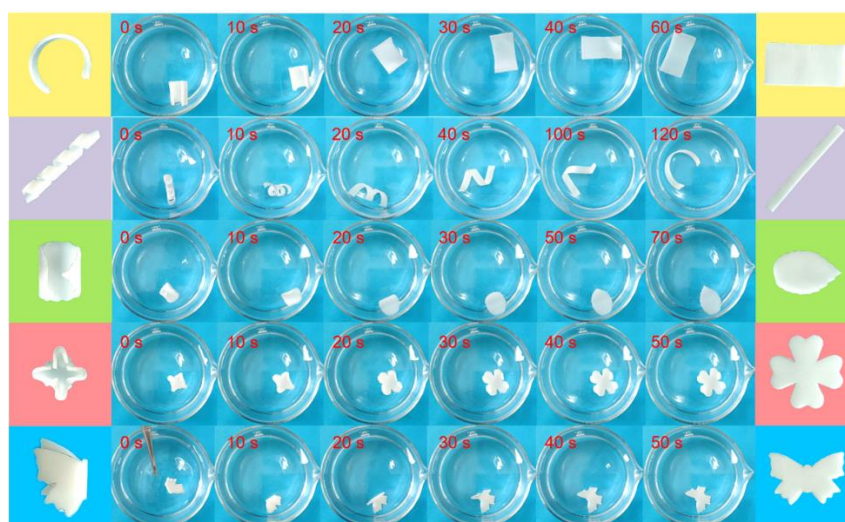
Figure S10. The shape recovery processes of PCLE-50% when heated by hot water of 60 °C.
