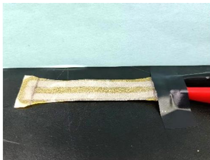
Figure S12. Specimen without pre-tension programming did not bend after heating, excluding the influence of differences in thermal expansion coefficients of materials.
