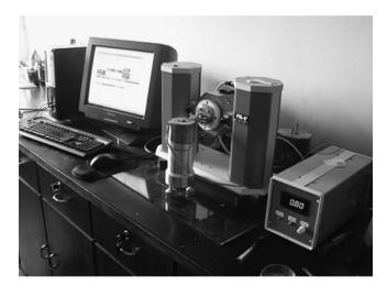
Fig. 2. Photograph of the modified DMA.
