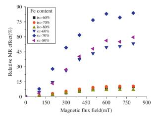
Fig. 4. Relationship between relative MR effect and magnetic flux field for isotropic (iso-) and structured (str-) MREs with different iron particle contents in the matrix at the frequency of 10 Hz.
