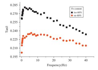
Fig. 5. Relationship between  $\tan \delta$  and frequency for isotropic (iso-) and structured (str-) MREs with the iron particle contents of 60%.
