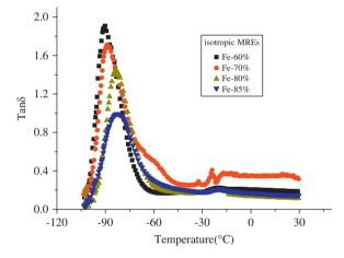
Fig. 1. Relationship between  $\tan \delta$  and temperature for isotropic MREs with different content of iron particles.
