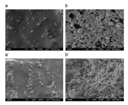
Fig. 3. The distribution of particles for isotropic (a and b) and structured (a' and b') MREs with the iron particle contents of 60% and 80% viewed by SEM.
