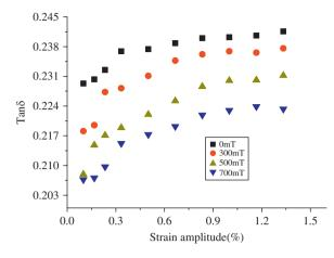
Fig. 6. Relationship between  $\tan \delta$  and strain at the different magnetic flux field for structured MREs with the iron particle contents of 70%.
