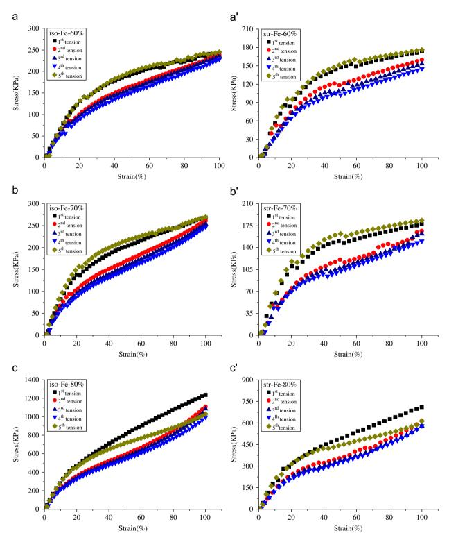
Fig. 7. Stress-softening effect of isotropic (iso-) and structured (str-) MREs with the iron particle contents of 60% (a, a'), 70% (b, b') and 80% (c, c'), respectively.
