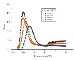
Fig. 2. Relationship between  $\tan \delta$  and temperature for structured MREs with different content of iron particles.
