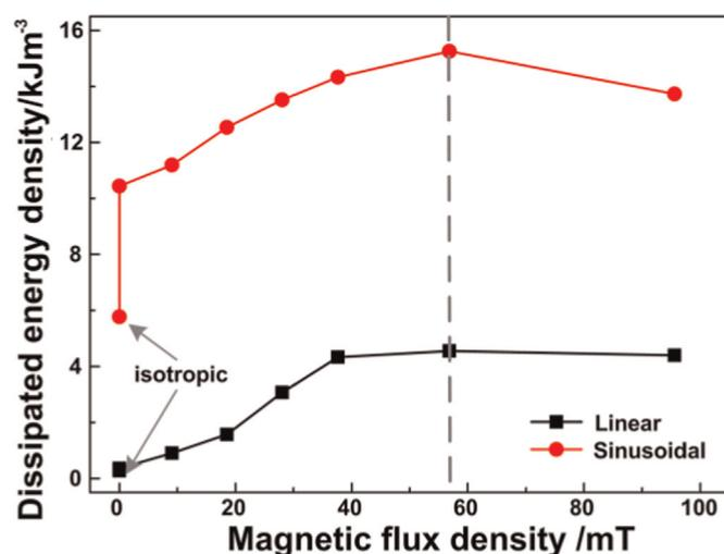
Fig. 2. The dissipated energy density of MRP-70 varies with different magnetic fields actuated by cyclic sinusoidal and linear strain, respectively. The MRP-70 is anisotropic except for the isotropic ones (marked as 'isotropic' in the figure).
