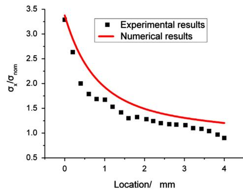
**Fig. 6.** Stress distribution of the numerical and the experimental method.
