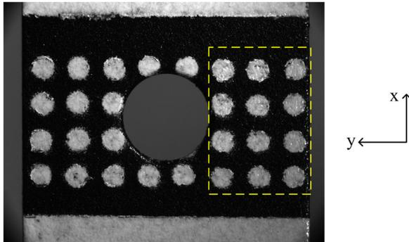
**Fig. 3.** Tensile specimen with traditional grid.
