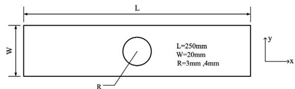
Fig. 2. Configuration of the specimens.
