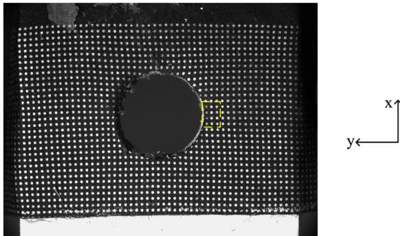
**Fig. 4.** Tensile specimen with new grid.
