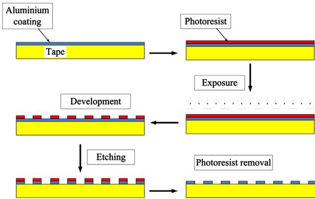
Fig. 1. Grid manufacturing process by lithography technique.
