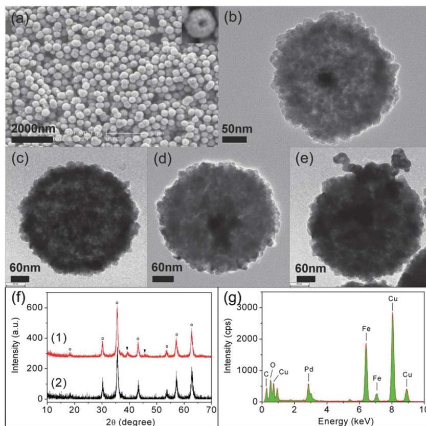
**Fig. 1** SEM and TEM images of the rattle type Pd@Fe<sub>3</sub>O<sub>4</sub> nanocomposites (a,b,d,e) and Fe<sub>3</sub>O<sub>4</sub> hollow spheres (c); XRD patterns of the rattle type Pd@Fe<sub>3</sub>O<sub>4</sub> nanocomposites (f1) and Fe<sub>3</sub>O<sub>4</sub> hollow spheres (f2); EDX spectra of the rattle type Pd@Fe<sub>3</sub>O<sub>4</sub> nanocomposites (g); Inset of (a) shows the SEM image of a typical broken rattle type Pd@Fe<sub>3</sub>O<sub>4</sub> microsphere.
