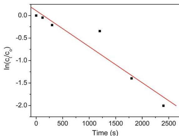
Fig. 6 The relative Plot of  $\ln(C_t/C_0)$  versus time with Ag@Fe<sub>3</sub>O<sub>4</sub> catalysts.
