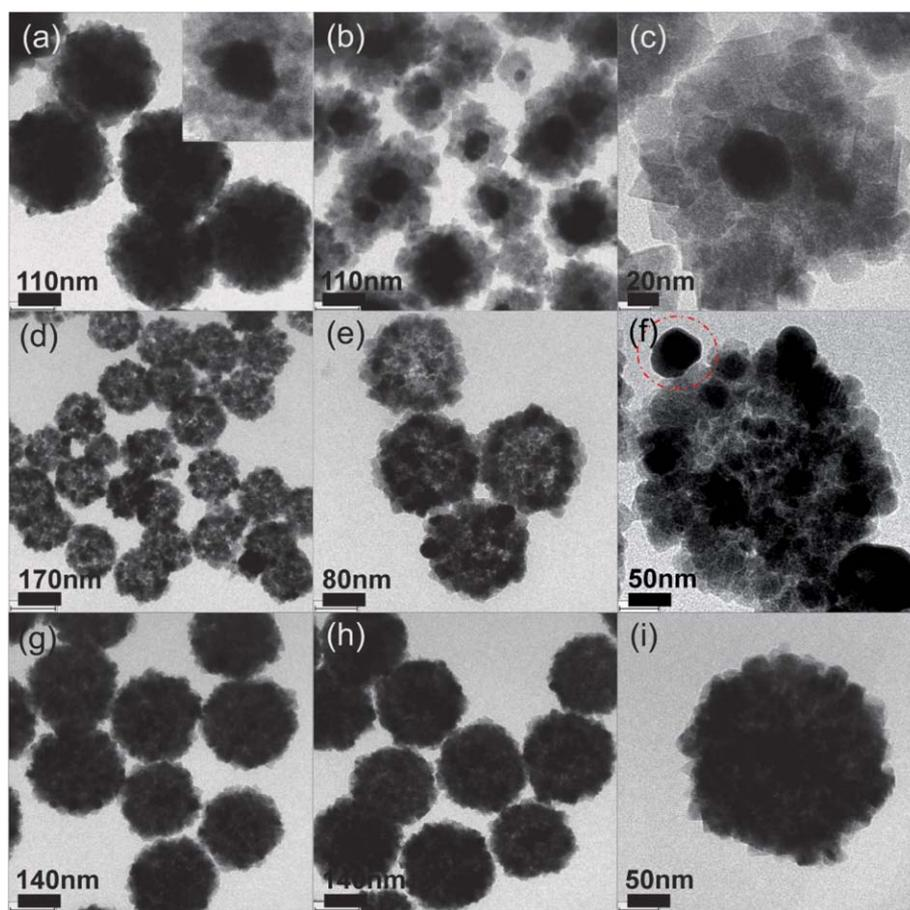
**Fig. 2** TEM images of the rattle type Ag@Fe<sub>3</sub>O<sub>4</sub> nanocomposites with different AgNO<sub>3</sub> concentrations:  $5 \times 10^{-3}$  M (a) and  $2.5 \times 10^{-2}$  M (b,c); TEM images of the Au/Fe<sub>3</sub>O<sub>4</sub> nanocomposites (d,e,f); and TEM images of the Cu<sub>0.1</sub>/Cu<sub>0.3</sub>Fe<sub>2.7</sub>O<sub>4</sub> nanocomposites (g) and Cu<sub>0.3</sub>Fe<sub>2.7</sub>O<sub>4</sub> hollow spheres (h,i).
