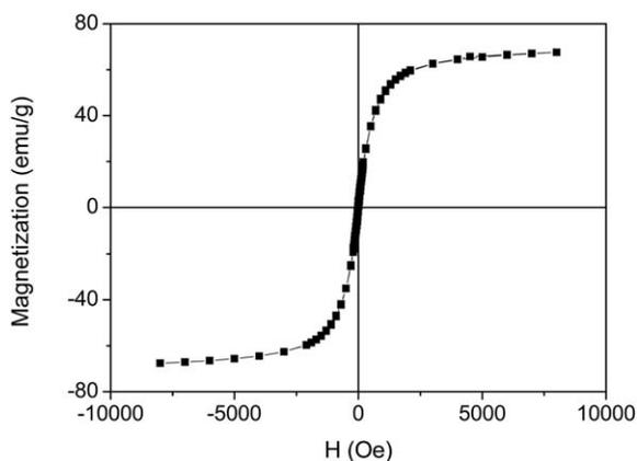
Fig. 4  $M-H$  (b) curve of the as prepared Pd@Fe<sub>3</sub>O<sub>4</sub>-2 rattle particles.
