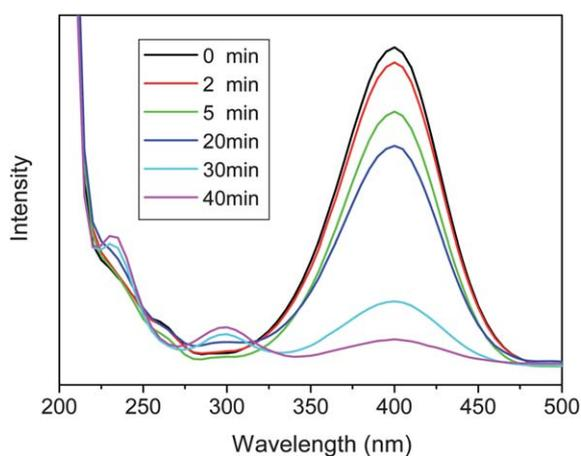
Fig. 5 Time-dependent UV-vis absorption spectral changes of the reaction mixture catalyzed by 200 nm Ag@Fe<sub>3</sub>O<sub>4</sub> nanocatalyst.
