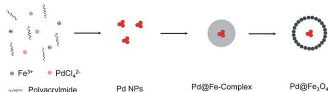
**Scheme 1** Schematic illustration of the formation of the rattle type nanostructure.
