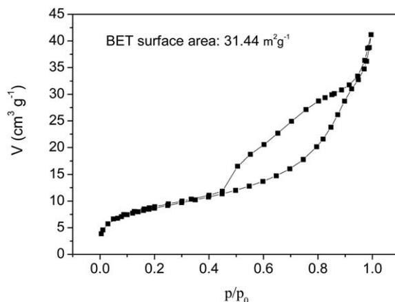
**Fig. 3** Nitrogen adsorption-desorption isotherm of the as prepared Pd@Fe<sub>3</sub>O<sub>4</sub>-2 rattle particles.
