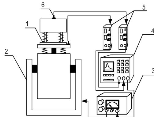
**Fig. 6** The set-up for evaluating the frequency-shift property. 1. SAVA 2. Vibration table 3. Power amplifier of the vibration table 4. Signal analyzer 5. Charge amplifier 6. Acceleration transducer
