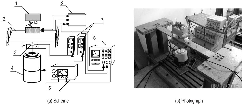
**Fig. 9** Experimental set-up for evaluating the vibration attenuation performance of the SAVA. 1. SAVA 2. Clamped-clamped beam 3. Impedance head 4. Exciter 5. Power amplifier of the exciter 6. Signal analyzer 7. Charge amplifier 8. Control system of the SAVA
