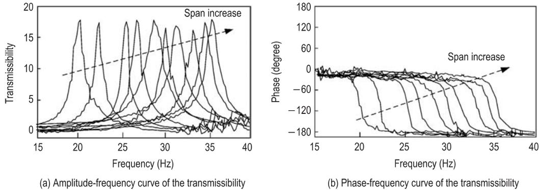
Fig. 7 The transmissibility versus frequency at various spans
