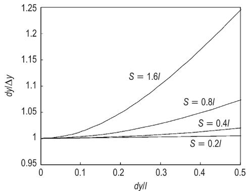
**Fig. 3** The ratios of exact and approximate deformation with different spans
