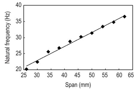
Fig. 8 The frequency-shift property of the SAVA. ♦ experimental data; —fitting curve
