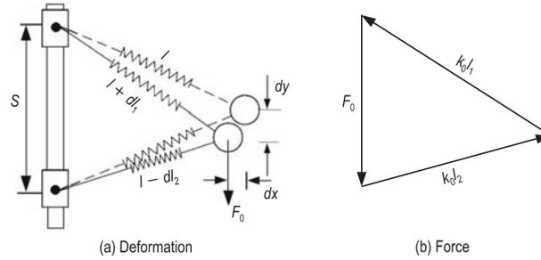
**Fig. 2** Deformation and force analysis of the SAVA
