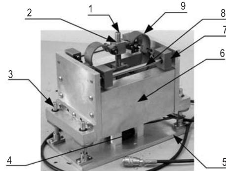
**Fig. 4** The photograph of the SAVA. 1. Screw rod 2. Screw cap 3. Vertical guide 4. Step motor 5. Base 6. Absorber mass 7. Horizontal slider 8. Horizontal guide 9. Leaf spring
