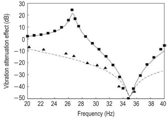
**Fig. 11** The vibration attenuation of absorbers.  $\blacktriangle$ SAVA (experimental data); - - - - -SAVA (numerical data);  $\blacksquare$  TVA (experimental data); —TVA (numerical data)
