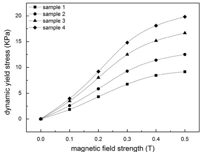
Fig. 7. Dynamic yield stresses as a function of the magnetic field for MR fluids containing different weight ratio of Fe nanowires.
