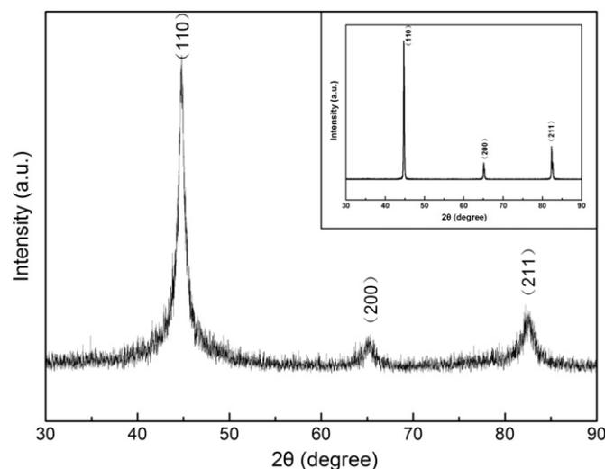
**Fig. 1.** XRD patterns of the Fe nanowires, the inset is the XRD patterns of CI.
