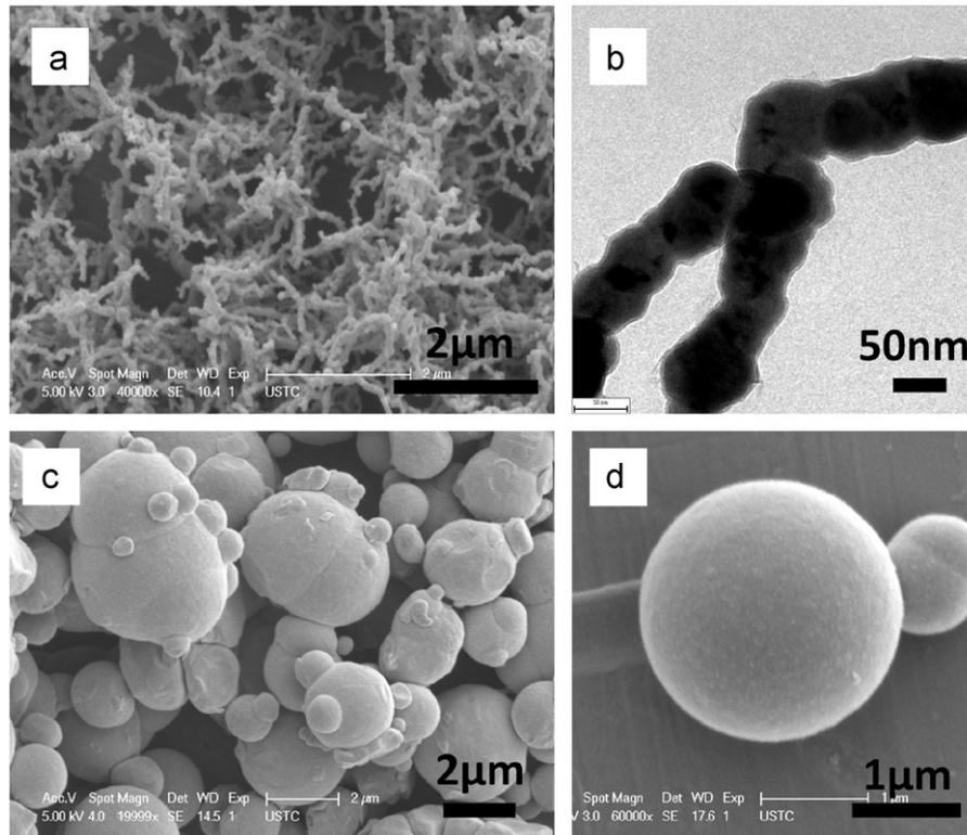
Fig. 3. SEM (a) and TEM (b) images of the wire-like Fe nanostructures, SEM (c,d) images of CI particles in different magnifications.
