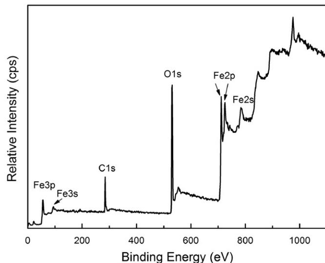
**Fig. 2.** XPS spectrum of the Fe nanowires.
