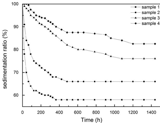
Fig. 8. Sedimentation percentages as a function of time for MR fluids containing different weight ratio of Fe nanowires.
