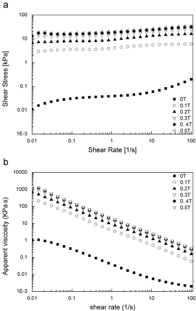
Fig. 5. (a) Flow curve (shear stress vs. shear rate) of MR fluid containing 6 wt% Fe nanowires (b) viscosity curve (viscosity vs. shear rate) of MR fluid containing 6 wt% Fe nanowires.
