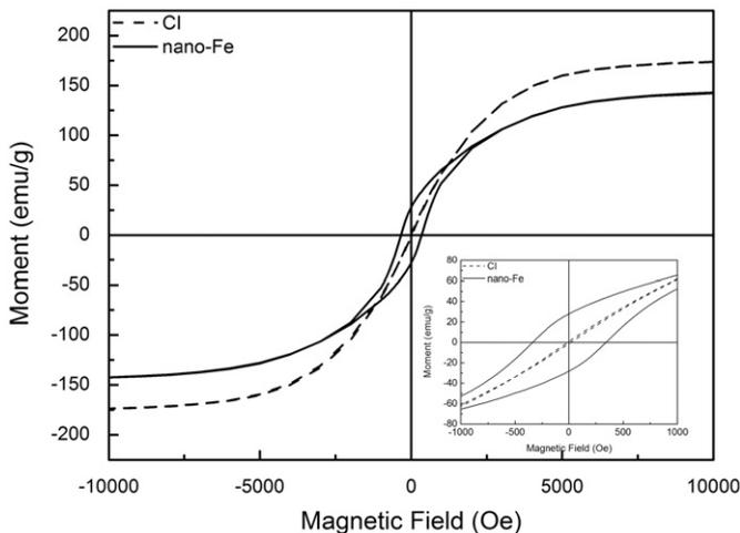
Fig. 4.  $M$ – $H$  curve of the nanowire Fe samples at 300 K.
