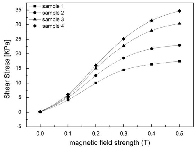
Fig. 6. Shear stresses as a function of the magnetic field for MR fluids containing different weight ratio of Fe nanowires.
