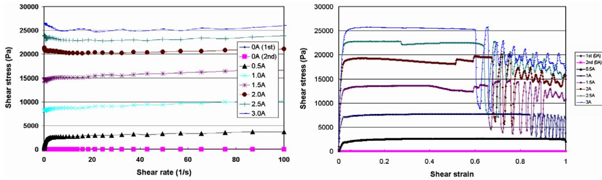
Figure 4. The steady shear and quasi-static shear results of the MRSTF sample based on 0% w/w STF.
