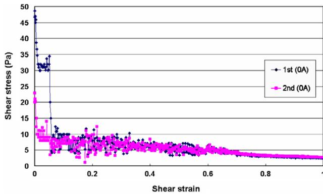
**Figure 8.** Quasi-static shear result of MRSTF based on 15% w/w STF.
