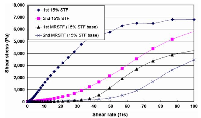
Figure 6. The steady shear results of the MRSTF sample based on 15% w/w STF and the STF sample.
