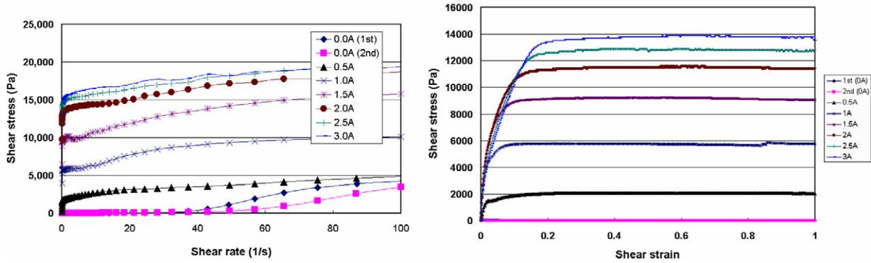
Figure 1. The steady shear and quasi-static shear results of the MRSTF sample based on 15% w/w STF.
