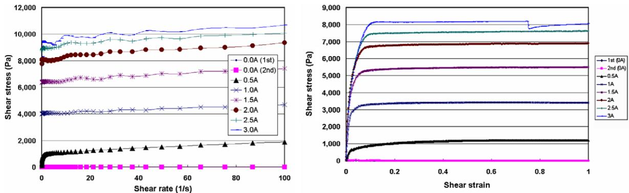
Figure 2. The steady shear and quasi-static shear results of the MRSTF sample based on 10% w/w STF.
