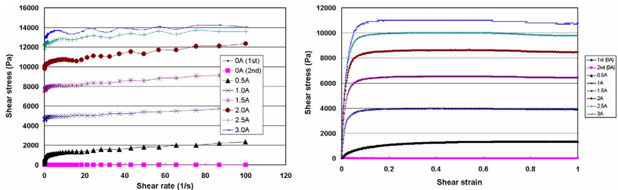
Figure 3. The steady shear and quasi-static shear results of the MRSTF sample based on 5% w/w STF.
