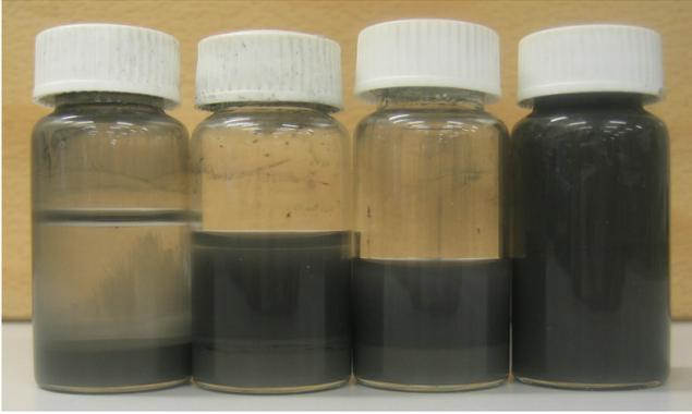
**Figure 7.** Particle settling testing with different weight fractions. A: 0%; B: 5%; C: 10%; and D: 15%.
