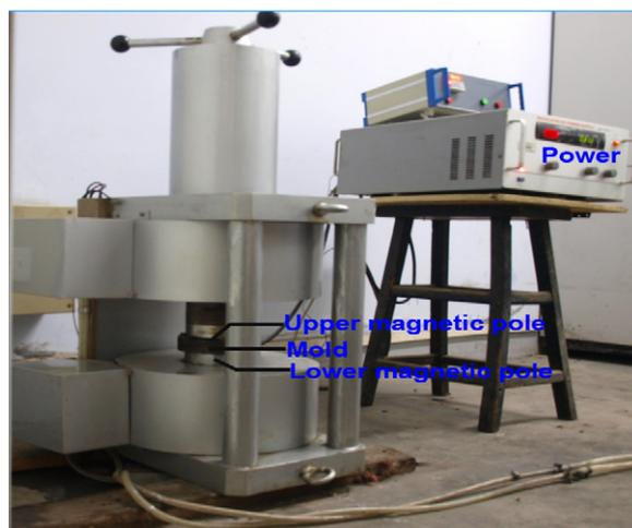
**Figure 1.** The magnetic field apparatus for *in situ* polycondensation. (This figure is in colour only in the electronic version)
