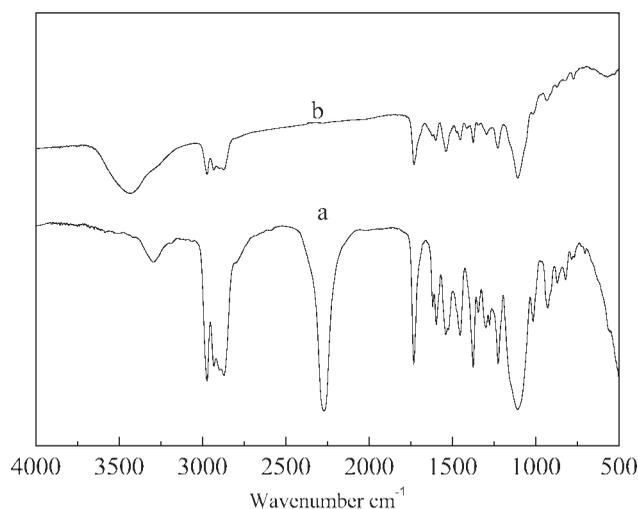
**Figure 1** FTIR spectra of the PU at different reaction time in the range  $500\text{--}4000 \text{ cm}^{-1}$ : (a) 30 min after reaction, (b) 3.5 h after reaction.
