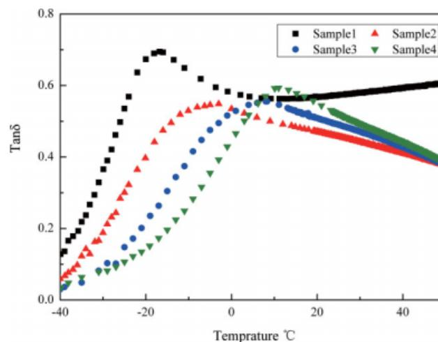
**Figure 8** Relationship between loss factor and temperature for different reaction molar ratio PU MREs. [Color figure can be viewed in the online issue, which is available at [www.interscience.wiley.com](http://www.interscience.wiley.com).]
