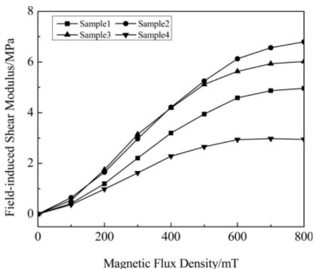
**Figure 4** Relationship between field-induced shear modulus and magnetic field for different reaction molar ratio PU MREs.
