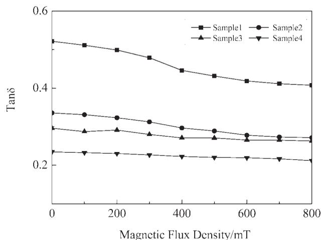
**Figure 7** Relationship between loss factor and magnetic field for different reaction molar ratio PU MREs.
