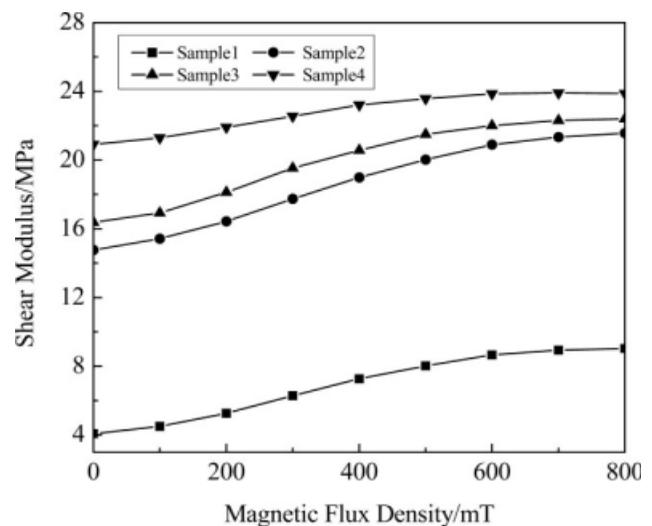
**Figure 3** The shear modulus of the samples for different reaction molar ratio PU MREs.
