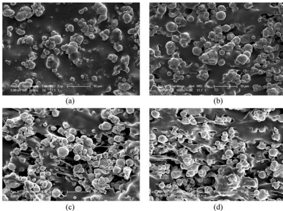
**Figure 2** The microstructure of the MRE based on polyurethane observed by SEM: (a) sample 1, (b) sample 2, (c) sample 3, and (d) sample 4.
