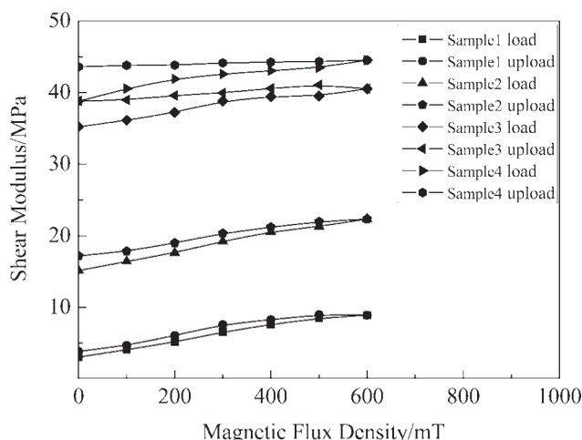
**Figure 6** Hysteresis loops of different NCO/OH ratio PU MREs under the magnetic field ranged from 0 to 600 mT.
