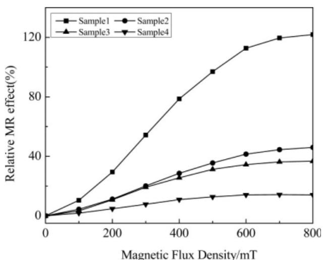
**Figure 5** Relationship between relative MR effect and magnetic field for different reaction molar ratio PU MREs.
