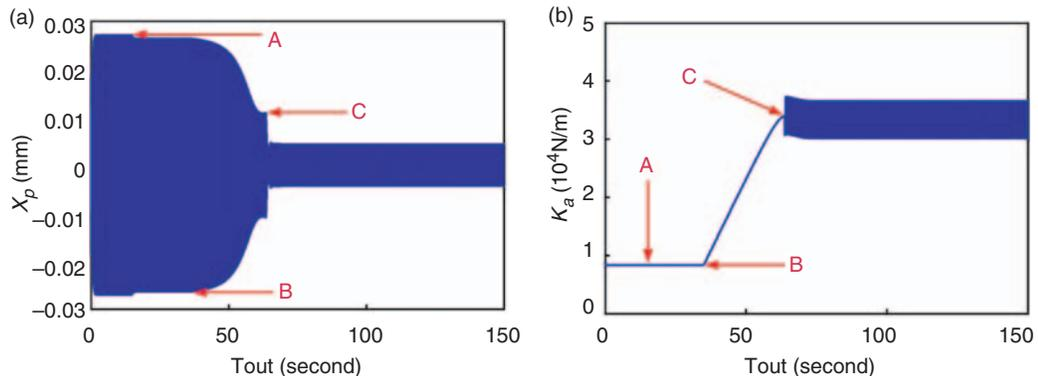
Figure 11. The simulation results of the proposed MRE-PZT DSTDVA with  $\alpha=0.1$ ,  $B=0.05$ : (a) the displacement of primary system; (b) the stiffness of DSTDVA.
