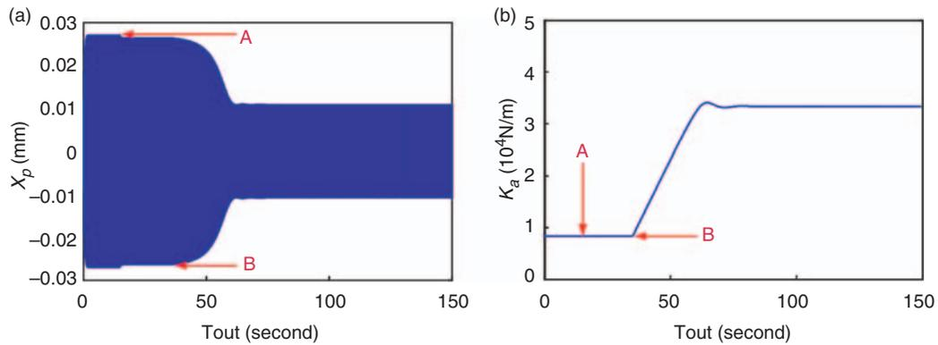
Figure 10. The simulation results of the conventional MRE-based quasi-static tuned ATVA: (a) the displacement of primary system; (b) the stiffness of ATVA.
