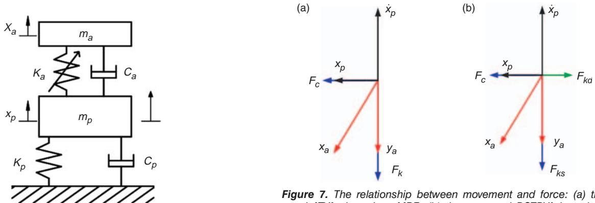
Figure 6. The scheme of the primary system with DVA.
