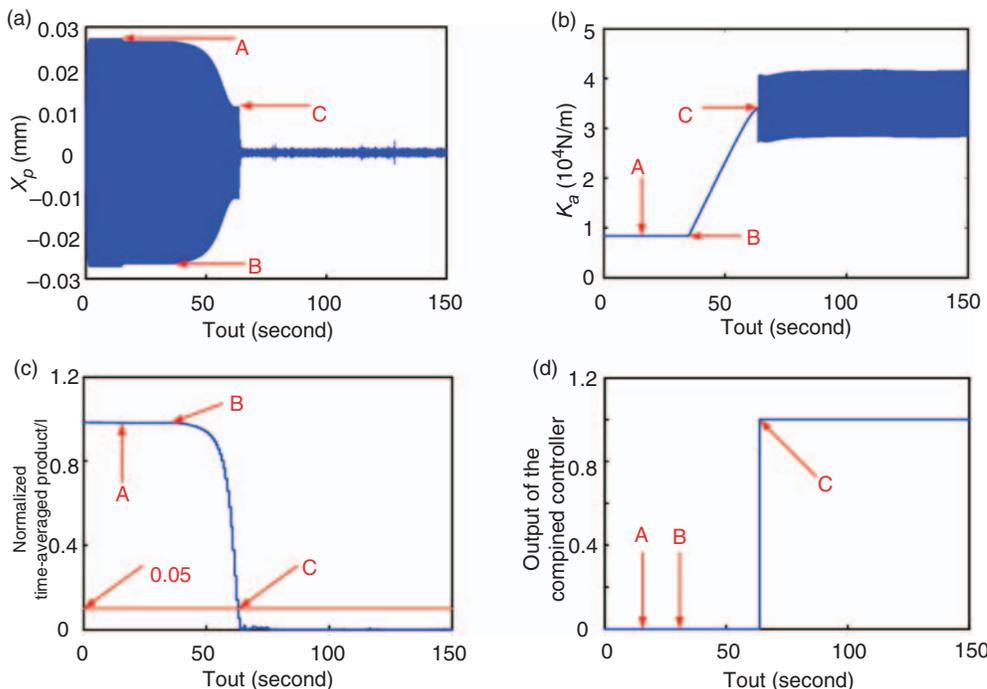
**Figure 9.** The simulation results of the proposed MRE-PZT DSTDVA with  $\alpha = 0.2$ ,  $B = 0.05$ : (a) the displacement of the primary system; (b) the stiffness of DSTDVA; (c) the normalized time-averaged product; (d) the output of the combined controller.
