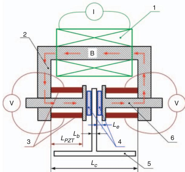
**Figure 3.** The scheme of the proposed DSTDVA 1. Excitation winding; 2. C-shape magnetic conductor; 3. Terrace PZT actuator; 4. MRE; 5. Base; 6. Moveable arm.
