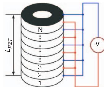
**Figure 4.** The scheme of terrace PZT actuator.
