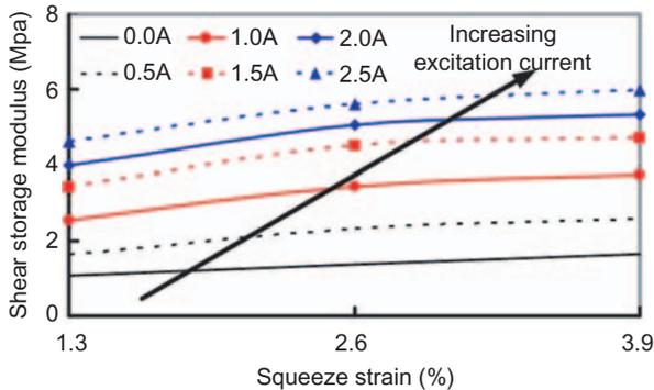
Figure 1. The shear storage modulus of MRE.
