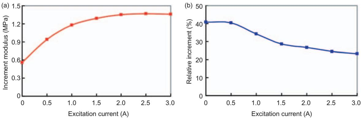
Figure 2. The detail enhanced effect of squeeze strain on shear storage modulus: (a) the increment  $\Delta G$ ; (b) the relative increment modulus  $\Delta G/G_{\epsilon=2.6\%}$ .
