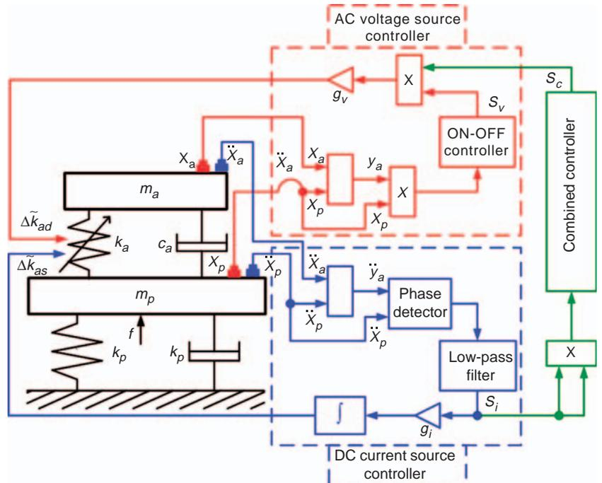
Figure 8. The control system of the proposed DSTDVA based on MRE.
