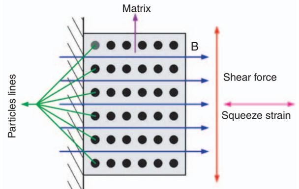
**Figure 5.** The directions of magnetic field, shear force, and squeeze strain.
