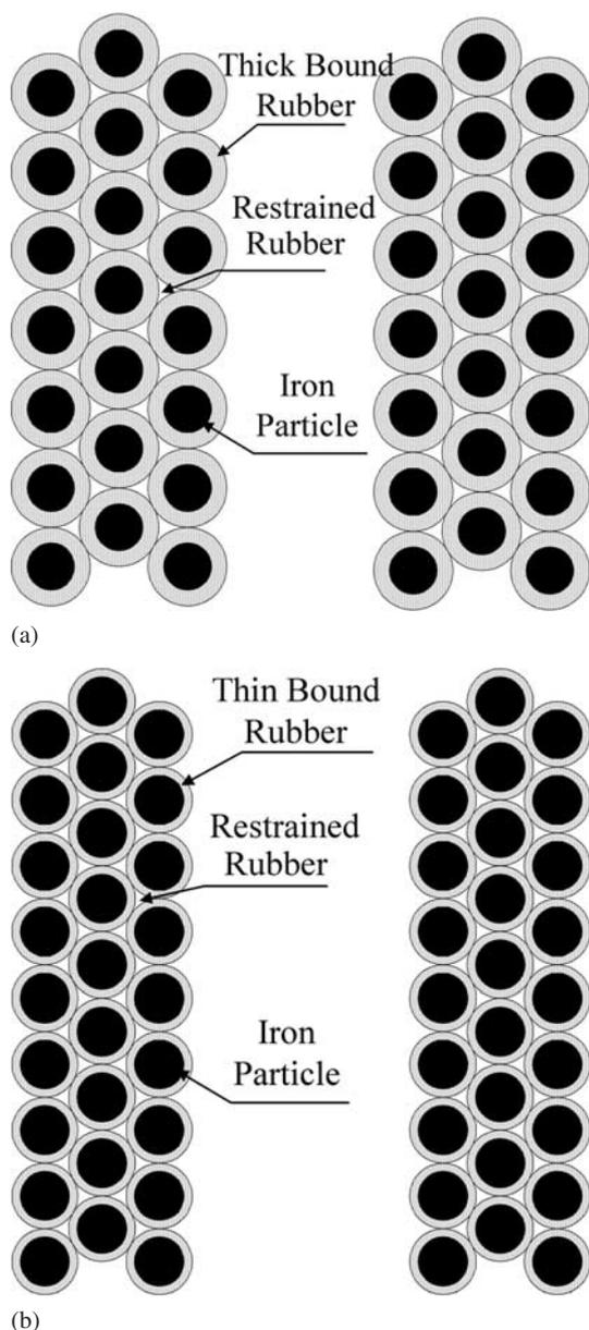
Fig. 9. Sketch of MRE's microstructure (a) MRE is prepared under low PS temperature: having thick bound rubber; (b) MRE is prepared under high PS temperature: having thin bound rubber.
