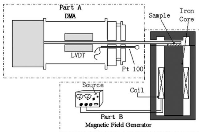
Fig. 2. Sketch of the modified DMA.
