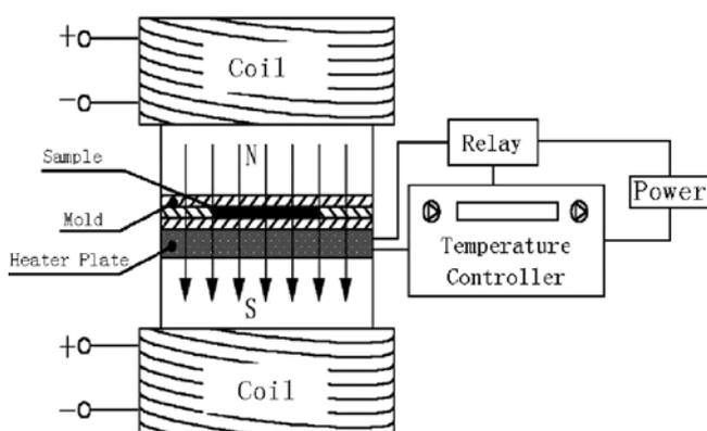
Fig. 1. Sketch of the PS device.
