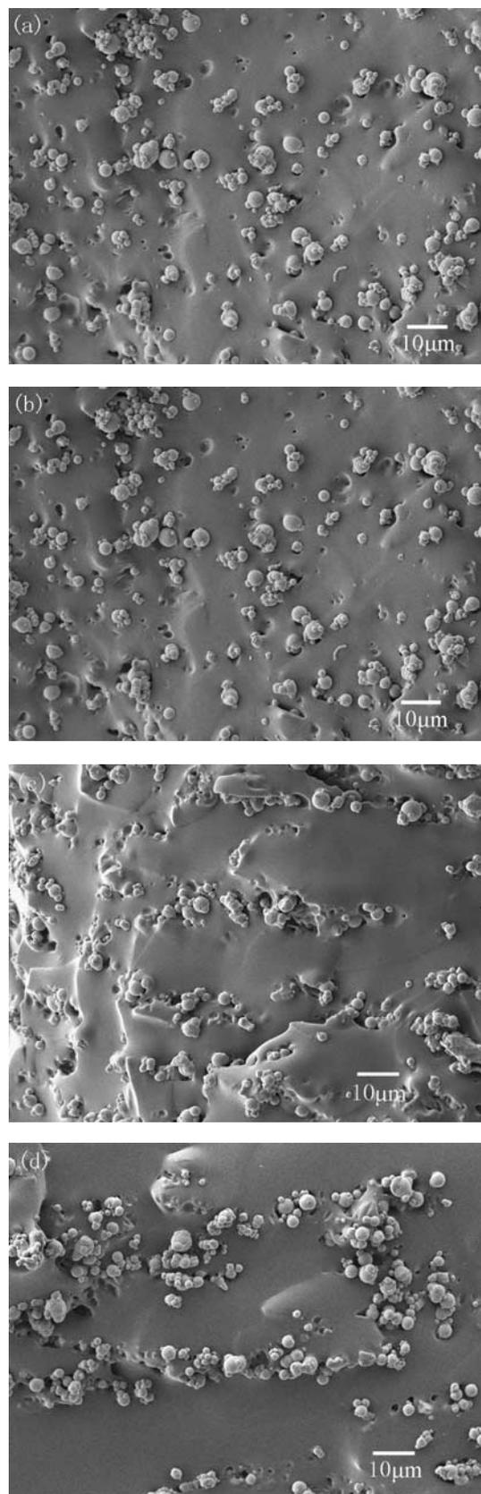
Fig. 5. SEM images of samples with different PS magnetic fields, (a) 0 mT, (b) 54 mT, (c) 110 mT, and (d) 350 mT.
