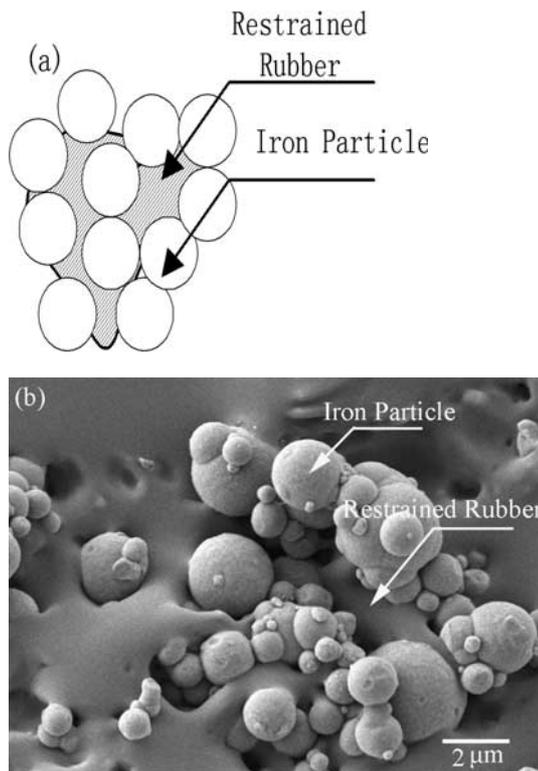
Fig. 4. Restrained rubber, (a) schematic diagram (b) SEM image.
