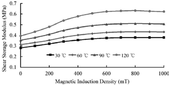
Fig. 7. Shear storage modulus of MRE samples prepared with different PS temperatures (PS magnetic field is 350 mT, PS time is 10 min).
