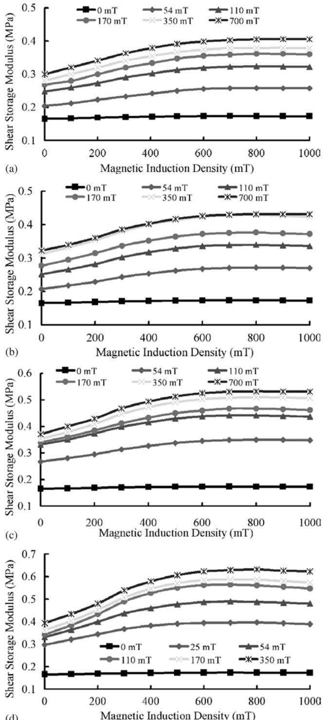
Fig. 8. Shear storage modulus of four groups of MRE samples whose PS temperature was (a) 30 °C, (b) 60 °C, (c) 90 °C and (d) 120 °C.
