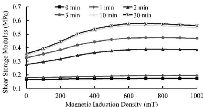
Fig. 6. Shear storage modulus of MRE samples prepared with different PS times (PS magnetic field 110 mT, PS temperature is 120 °C).
