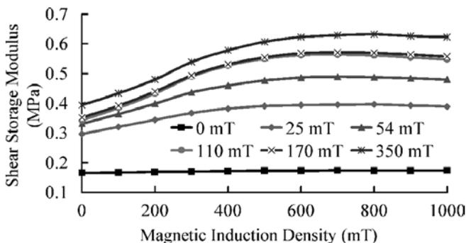
Fig. 3. Shear storage modulus of MRE samples prepared with different PS magnetic field (PS temperature is 120°C, PS time is 10 min).
