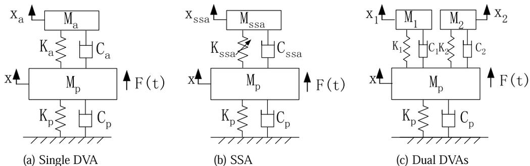
Fig. 3. Single DVA, SSA and dual DVAs mounted on identical primary systems.
