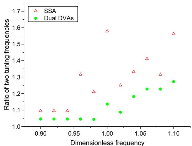
Fig. 5. Ratio of two tuning frequencies in SSA and dual DVAs.
