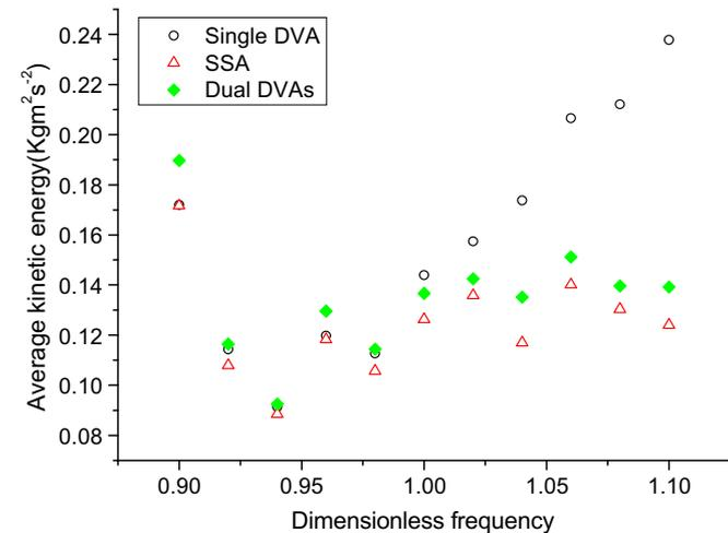
Fig. 4. Performance comparison of a single DVA, SSA and dual DVAs.
