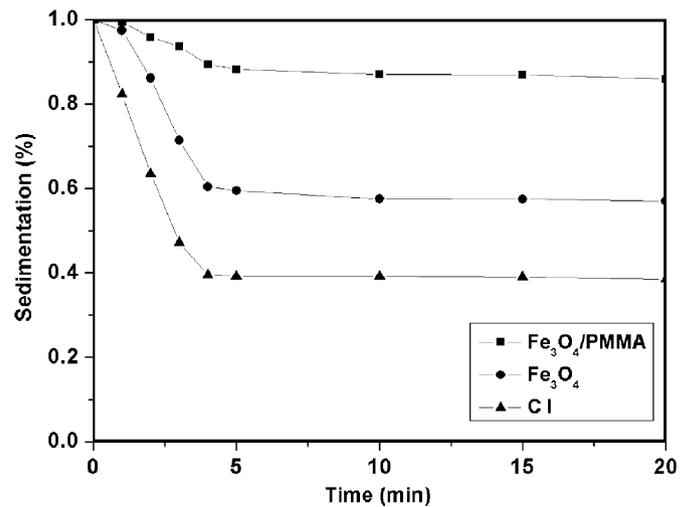
Fig. 5. Sedimentation ratio vs. time for MRFs of composite particles, magnetite and carbonyl iron.
