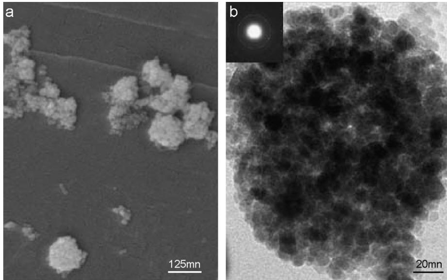
Fig. 2. (a) SEM and (b) TEM images of  $\text{Fe}_3\text{O}_4/\text{PMMA}$ , the insert is the electronic diffraction of a composite particle.
