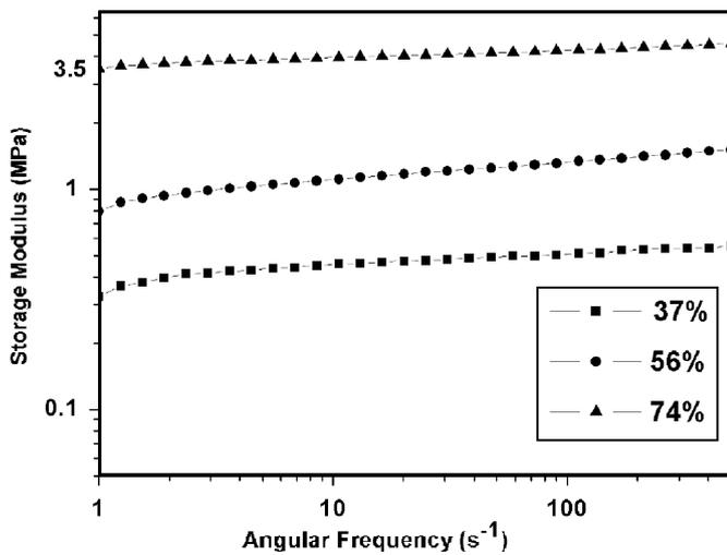
Fig. 4. Storage modulus as a function of angular frequency of different concentrations.
