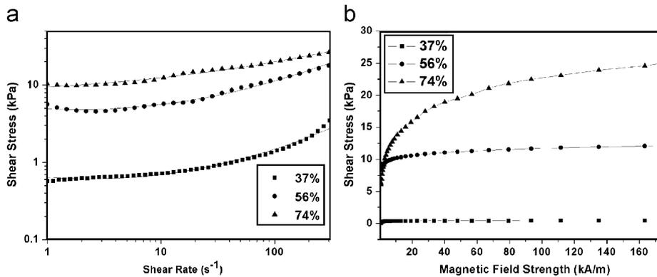
Fig. 3. Shear stress as a function of (a) shear rate and (b) magnetic field strength.
