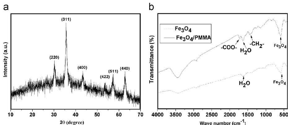
Fig. 1. (a) XRD patterns of Fe<sub>3</sub>O<sub>4</sub>/PMMA; (b) FTIR of Fe<sub>3</sub>O<sub>4</sub> and Fe<sub>3</sub>O<sub>4</sub>/PMMA.
