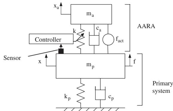
Fig. 4. A single-d.o.f. primary system with an AARA.
