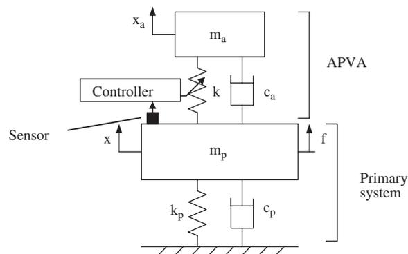
Fig. 1. A single-d.o.f. primary system with an APVA.
