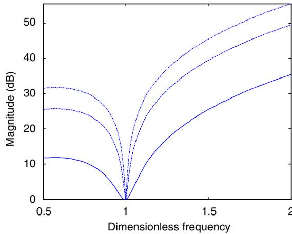
Fig. 2. Influence of the damping ratio  $\xi_a$  on  $|Z_a/Z_{PVA}|$ . Solid line:  $\xi_a = 0.05$ ; dashed line:  $\xi_a = 0.01$ ; and dash-dot line:  $\xi_a = 0.005$ .
