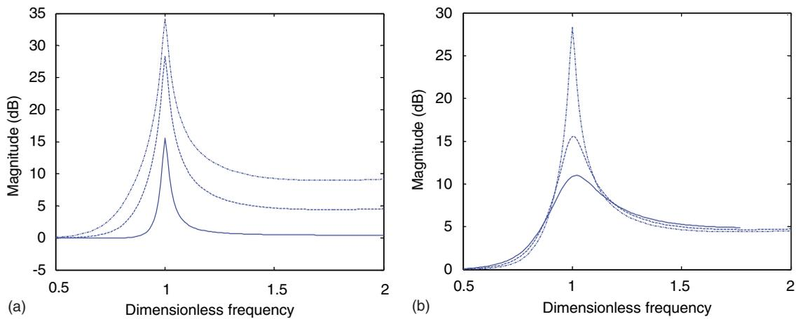
Fig. 3. Vibration reduction effect comparison: (a) the case APVA with different damping ratio,  $\mu = 0.01$ ,  $\xi_p = 0.01$ , solid line:  $\xi_a = 0.005$ ; dashed line:  $\xi_a = 0.01$ ; dash-dot line:  $\xi_a = 0.005$ ; and (b) the case primary system with different damping ratio,  $\mu = 0.01$ ,  $\xi_a = 0.01$ , solid line:  $\xi_p = 0.1$ ; dashed line:  $\xi_p = 0.05$ ; dash-dot line:  $\xi_p = 0.01$ .
