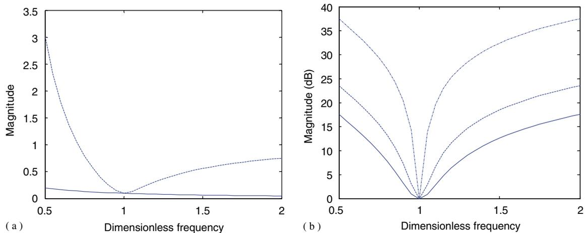
Fig. 5. Vibration control effort comparison: (a) the amplitude ratios of the control force and exciting force: solid line: AARA; dashed line: ARA; and (b) the amplitude ratios of the control force of AARA and ARA: solid line:  $\xi_a = 0.1$ ; dashed line:  $\xi_a = 0.05$ ; dash-dot line:  $\xi_a = 0.01$ .
