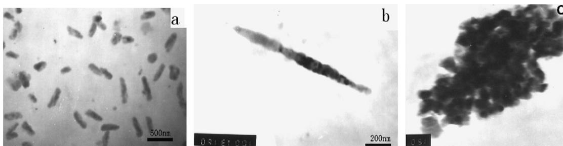
Fig. 6. (a) TEM image of  $\text{Ba}_{0.8}\text{Sr}_{0.2}\text{TiO}_3$  nanorods which was prepared by ultrasonic radiation for 20 min and heat-treated for 12 h at  $600^\circ\text{C}$ . (b) The magnified image. (c) TEM image of  $\text{Ba}_{0.8}\text{Sr}_{0.2}\text{TiO}_3$  nanorods which were heat-treated for 12 h at  $600^\circ\text{C}$  without ultrasonic radiation.
