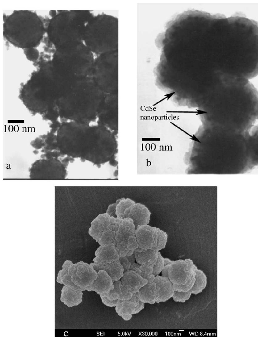
Fig. 6. TEM micrographs of SiO<sub>2</sub>@CdSe core-shell particles (a), SiO<sub>2</sub>@CdSe/PPy composite spheres (b) and SEM image of SiO<sub>2</sub>@CdSe/PPy composite spheres (c).
