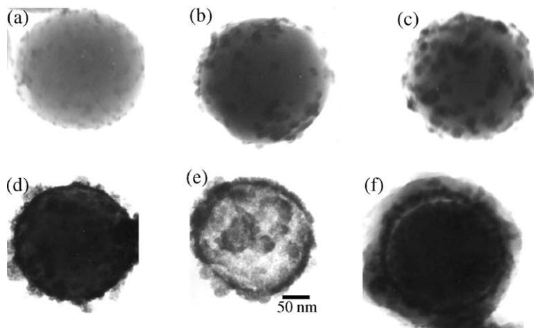
Fig. 4. TEM micrographs of spheres during the successive synthesis steps. A scale bar is 50 nm which corresponds to all photos. SiO<sub>2</sub>-CdSe composite samples 1–4 (a)–(d), CdSe hollow capsule (e), SiO<sub>2</sub>@CdSe /PPy composite sphere (f).
