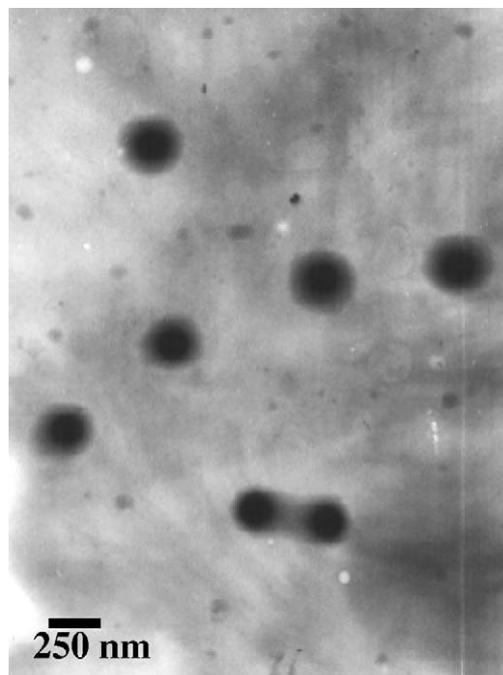
Fig. 2. TEM micrograph of  $\text{SiO}_2$  spheres encompassed by PVP macromolecules.
