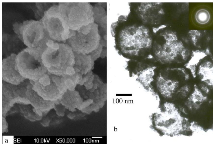
Fig. 9. SEM (a) and TEM (b) micrographs of CdSe hollow capsules.
