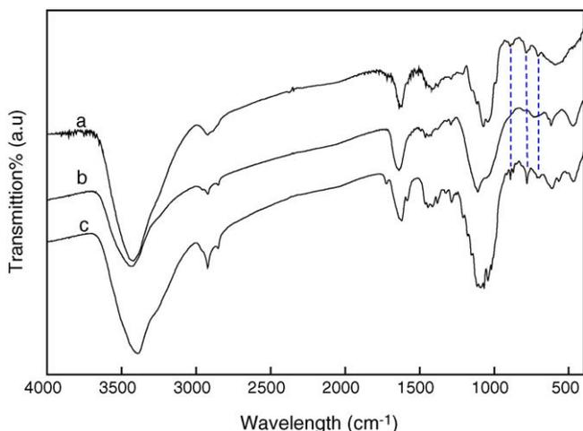
Fig. 10. FTIR spectra of doxorubicin (a), CdSe capsules (b) and CdSe capsules carrying doxorubicin (c).
