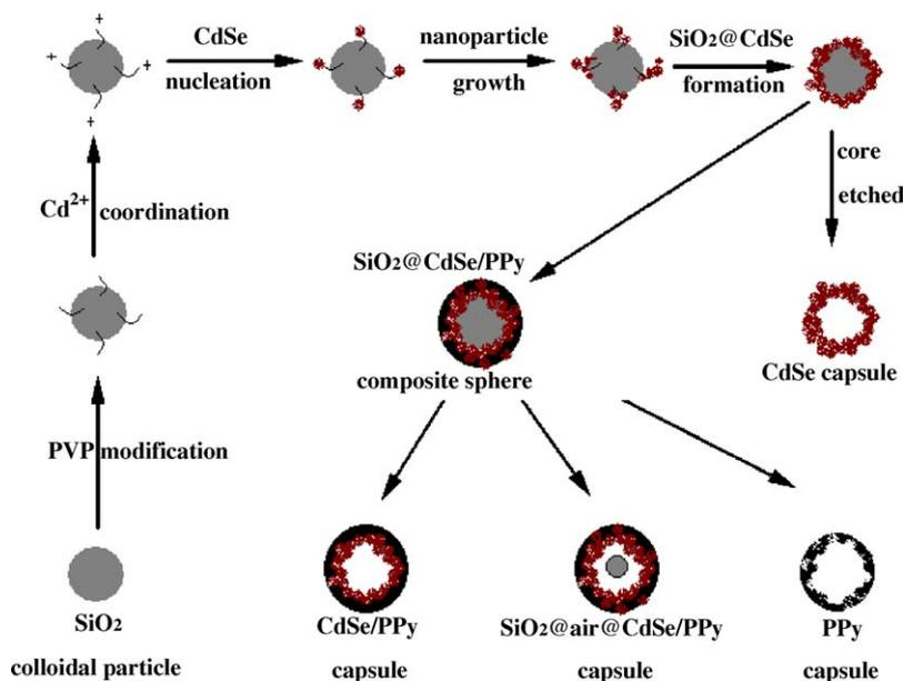
Fig. 1. Schematic diagram of the procedure for synthesizing core-shell particles and capsules.
