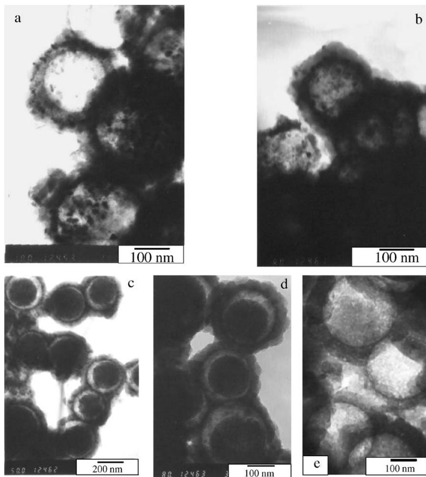
Fig. 12. TEM micrographs of CdSe/PPy (a, b), SiO<sub>2</sub>@air@CdSe/PPy (c, d) and mesoporous polypyrrole (e) capsules.
