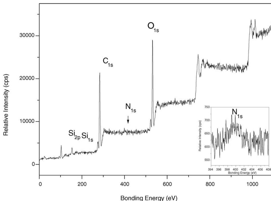
Fig. 3. XPS spectrum of PVP modifying  $\text{SiO}_2$  spheres.
