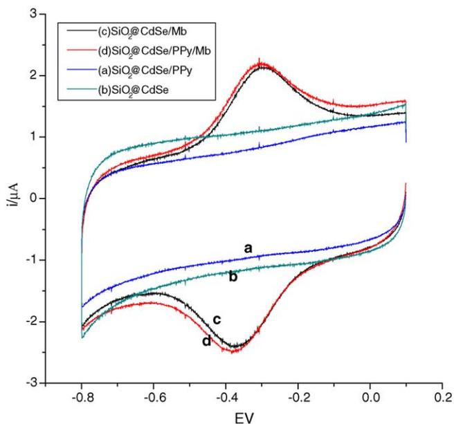
Fig. 8. Cycle voltammograms at scan rate  $0.2\text{ V s}^{-1}$  in pH 7.0 buffer for  $\text{SiO}_2\text{@CdSe}$  monolayer film (a),  $\text{SiO}_2\text{@CdSe-Mb}$  film (b),  $\text{SiO}_2\text{@CdSe/PPy}$  monolayer film (c) and  $\text{SiO}_2\text{@CdSe/PPy-Mb}$  film (d).
