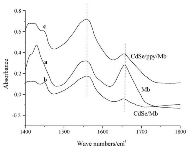
Fig. 7. RAIIR spectra of Mb (a),  $\text{SiO}_2\text{@CdSe-Mb}$  (b) and  $\text{SiO}_2\text{@CdSe/PPy-Mb}$  (c) films.
