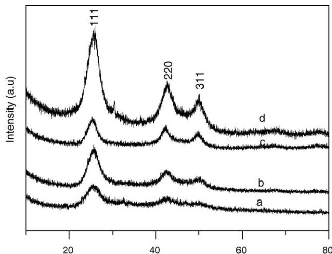
Fig. 5. X-ray diffraction patterns of SiO<sub>2</sub>-CdSe composite samples 1–4 (a)–(d).
