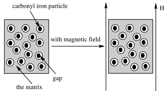
Fig. 5. The sketch of mechanism of MR elastomers with poor interaction between magnetic particles and matrix under magnetic fields.
