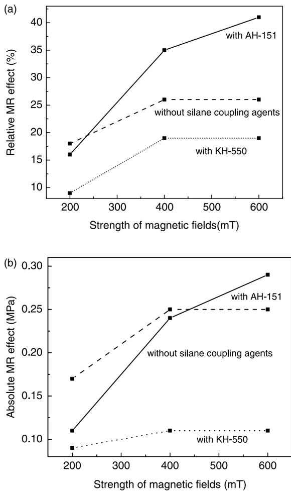
Fig. 3. Relative (a) and absolute (b) MR effect of MR elastomers with and without silane coupling agents as a function of strength of magnetic fields.
