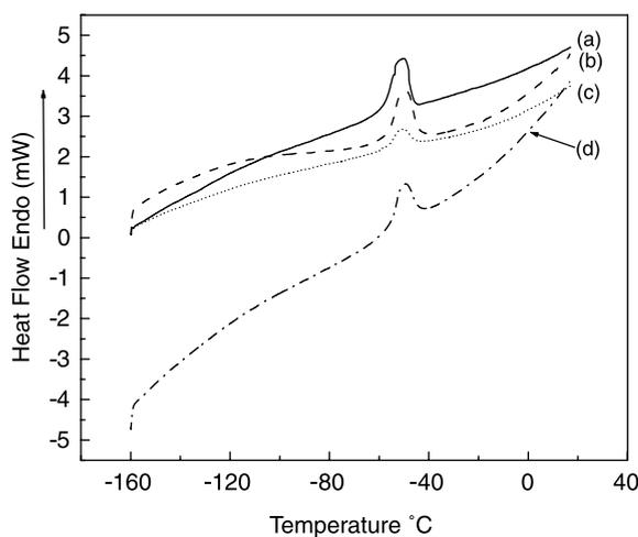
Fig. 2. DSC curves of MR elastomers without and with different silane coupling agents: (a) pure MVQ; (b) MVQ/Fe without modification; (c) MVQ/Fe/KH-550; (d) MVQ/Fe/AH-151.
