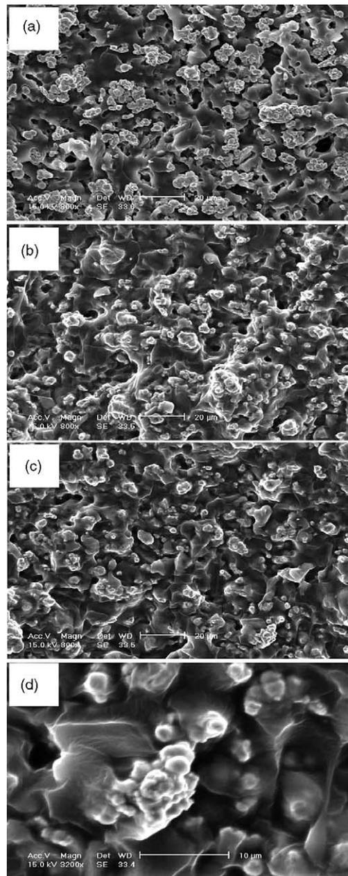
Fig. 1. SEM microstructure of MR elastomers (a) without silane coupling agents (b) with KH-550 (c) with AH-151 (d) magnification of (c).
