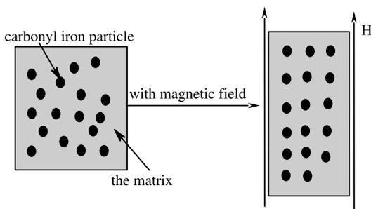
Fig. 4. The sketch of mechanism of MR elastomers under magnetic fields.
