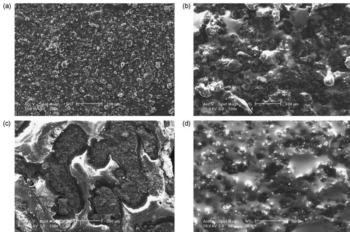
Fig. 4. SEM micrographs for MR elastomers prepared with different weight ratio of PU/Si-rubber: (a) 0/1, (b) 1/1, (c) 2/1, (d) 1/0, respectively.
