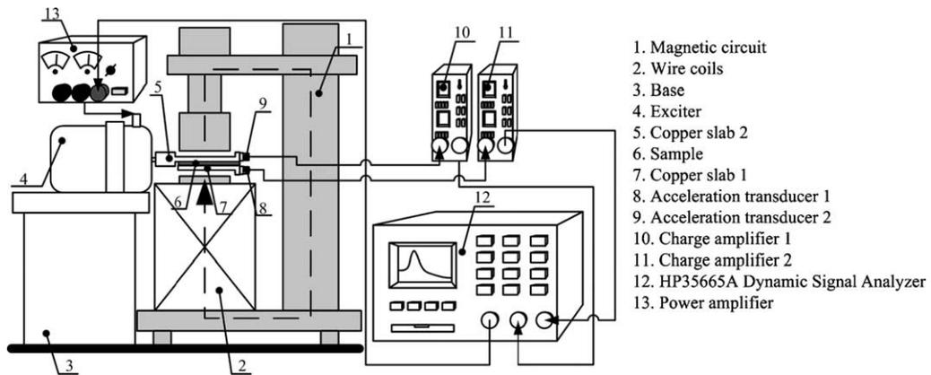
Fig. 1. Sketch of the measurement apparatus for MR elastomers.
