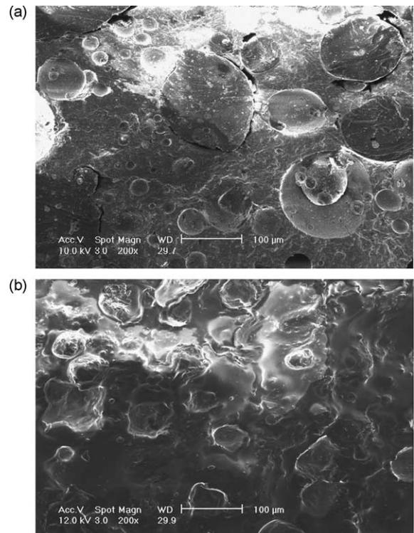
Fig. 3. SEM micrographs of PU/Si-rubber hybrid (a) without or (b) with Si-oil additive (weight ratio for all PU/Si-rubber hybrids is 1/1).
